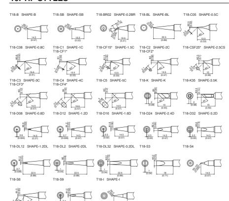
\* Tinned on the soldering surface only.
