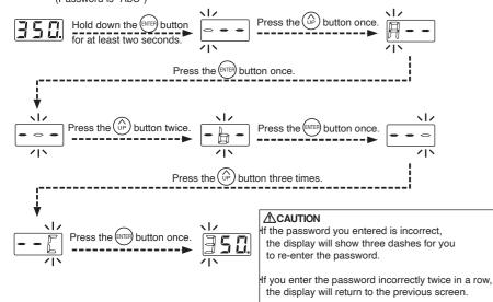
The unit will move to the change setting screen for each mode after entering the password. Please change the setting for each mode according to the procedure. (In the above example, please refer to the procedure for setting the temperature.)
