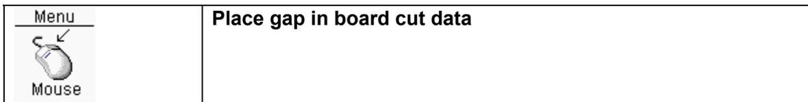
In the next dialogbox the gap length can be entered. After pressing the **OK** button the selected and concatenated two milling lines will be made shorter.
