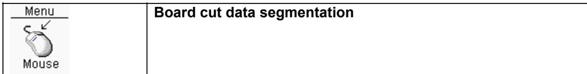
In the next dialogbox the gap and segmentation length can be entered. After pressing the **OK** button the selected milling line will be segmented.
